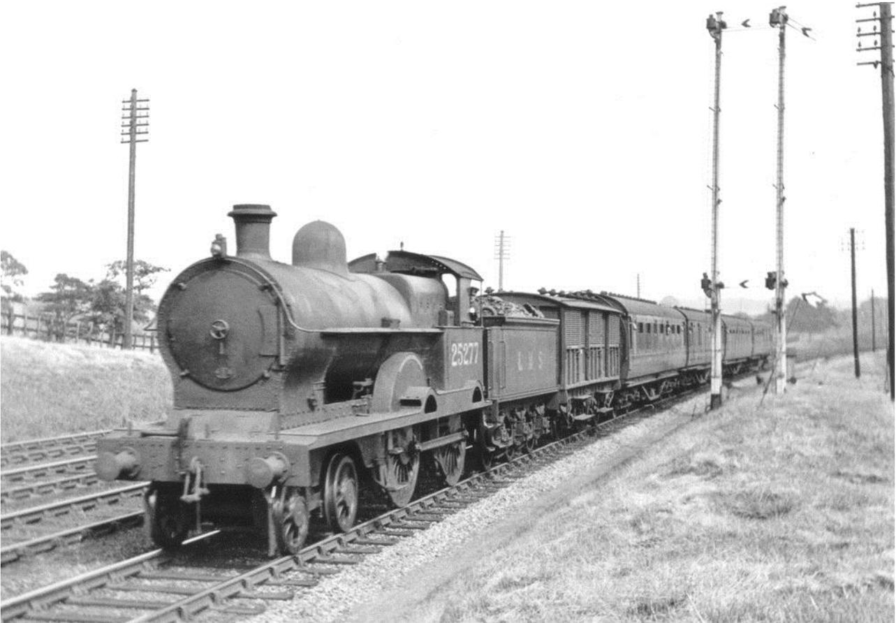
*An example of milk churns conveyed by an Ordinary Passenger train. Ex-LNWR Precursor Class 4-4-0 No.25277 Oberon at Whitrope, ten miles south of Crewe, on July 3<sup>rd</sup> 1937 with a secondary 4-set and an ex-North Staffordshire Railway 6w milk van behind the tender. ER MORTEN.*
